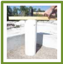
Figure 3: Hammering Pipe Into Media
