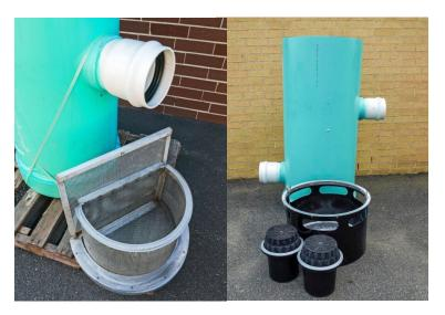
There are no hard and fast rules regarding cleaning frequency. The fact is installation sites (roofs) with higher-than-expected sediment loads require more maintenance. In general, Fabco Industries recommends cleaning DownSpout Filter units when the removable cartridge basin or screen basket becomes about one-third full, or if inlet/outlet pipes are obstructed.
