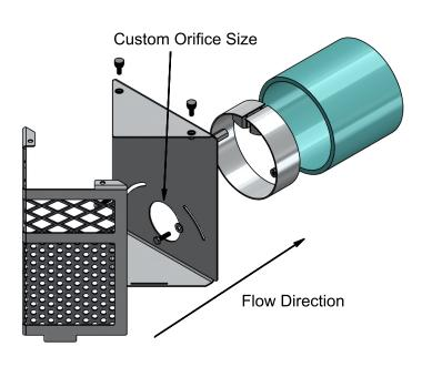
The expanding ring goes into the outlet pipe opening, and allows you to torque a bolt until the ring is tightly secured onto the pipe. Then the back plate can be installed onto the expanding ring and the front cover be placed on and secured with two thumb screws. The expanding ring requires no power tools or drilling of existing structures, making maintenance easy.
