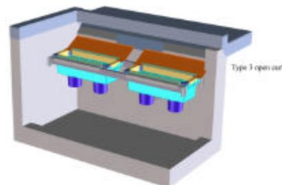
To accommodate the length of the two StormBasins and the increased length of the vault a unique fitting kit (P/N 9791-5D-000) is supplied for the Type 3 design.
